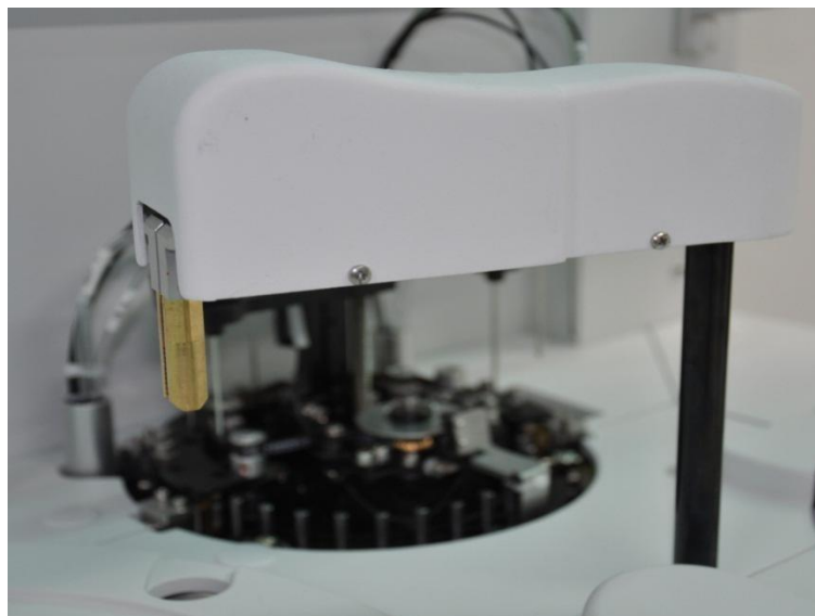
Figure 6.2.6 Transfer arm module
