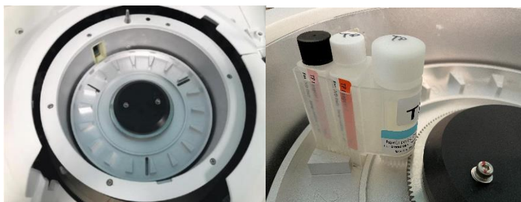
Figure 6.2.2 Reagent carousel and reagent bottles
