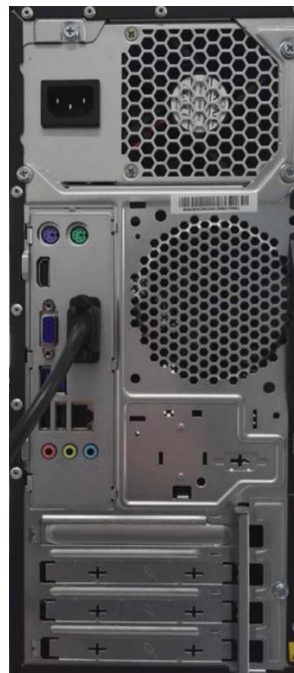
Figure 5.2.2 Communication port on computer
