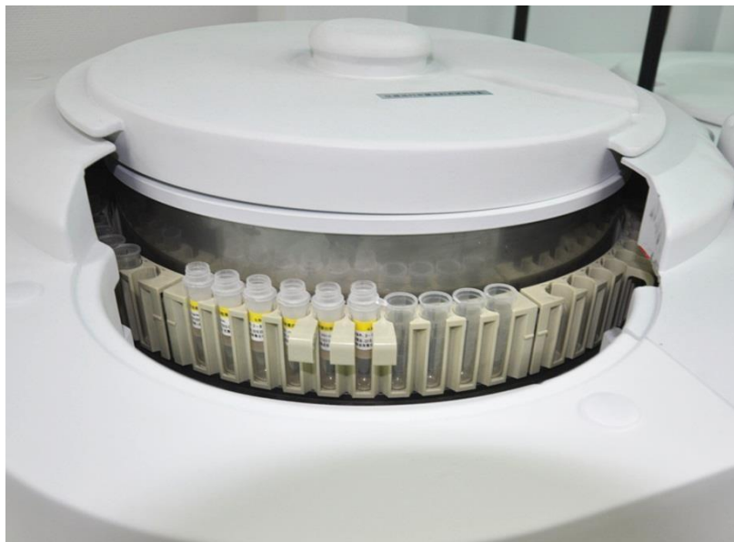
Figure 6.2.1 Sample rack and sample vessels
