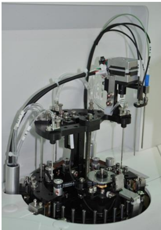
Figure. 6.2.7 Washing carousel and substrate needle
